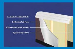
Finally, we have a Polyisocyanurate Reflective Silver Foil Wrap fitted to the inside of the cabinet and another 1" Polyurethane Foam Panel on the inside of the Silver Foil.
